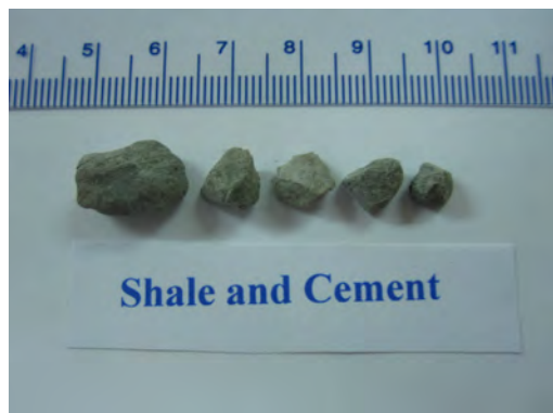
Fig. 4: The third fragment from left is a failed casing cement fragment. The rest are shale fragments.
