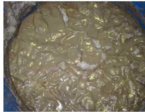
Fig. 2: Material received from the operator as collected from the choke and separator. The salt content is in excess of 250,000PPM
