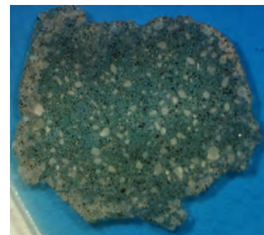
Fig. 3: Thin section of a failed casing cement recovered from the choke.
